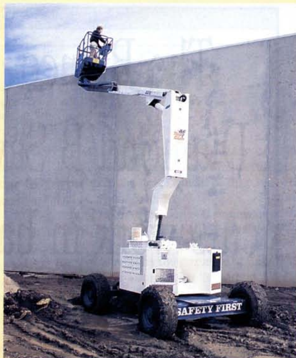
THE JLG "TOP-GUN" 40HA Articulated Boom: JLG's latest addition to the "Top-Gun" range. A go-anywhere, do anything machine designed for very rough terrain use. It has 2-wheel drive, zero tail-swing for tight corners and a powerful 28 HP Kubota diesel engine. Capacity (unrestricted) is 227 kg (500 lbs). Horizontal reach is 7.24 m (23 ft) and a maximum working height of 14.02 m (46 ft)
