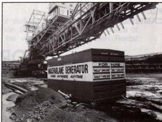
Macfarlane's 500kVA generator on-site at the Yallourn open-cut
