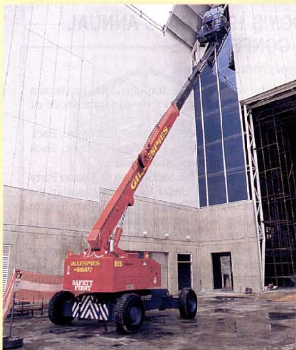
THE JLG 110HX: Large scale machines are often imported from JLG's American parent. This JLG 110HX, which has an unrestricted capacity of 227 kg (500 lbs) and a maximum capacity of 454 kg (1000 lbs) at full stretch, is able to put men and materials to work 33.5 m (110 ft) above the ground. It was re-engineered in Australia to have a special glass fixing platform and a wind velocity meter to warn of hazardous wind conditions.
